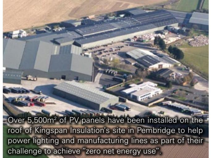
Over 5,500m<sup>2</sup> of PV panels have been installed on the roof of Kingspan Insulation's site in Pembridge to help power lighting and manufacturing lines as part of their challenge to achieve "zero net energy use".
